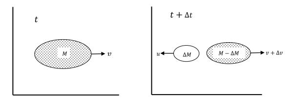
Consider a system of mass M moving with velocity v as shown in figure. After a time  $\Delta t$ , a mass  $\Delta M$  is ejected from the system with velocity u. As a result, mass of the system is reduced to  $(M - \Delta M)$  and its velocity increased to  $(v + \Delta v)$ .
