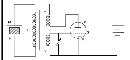
As shown in figure, X-cut slab of the Quartz crystal is placed between two metal plates M and N. These metal plates are connected to the coil L. Coil  $L_1$  is connected to the plate circuit while coil  $L_2$  is connected to tank circuit. Frequency of the plate circuit can be adjusted with the help of a variable capacitor C. When the frequency of plate circuit is equal to the natural frequency of the rod, resonance occurs and ultrasonics are produced.
