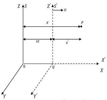
Consider two inertial frames of reference S, S'. Frame S' is moving with a velocity v along the positive X-axis relative to the frame S. Let the two frames of reference S, S' coincide at time t = 0.
