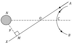
Consider an alpha particle or mass m and charge +2e moving towards a nucleus of charge +Ze in AX direction. Alpha particle follows a hyperbolic path ACB instead of a straight path AX due to coulomb's repulsion of the nucleus. p is the perpendicular distance from nucleus N to the initial direction of alpha particle. This is known as Impact parameter. Hence Impact parameter can be defined as follows.
