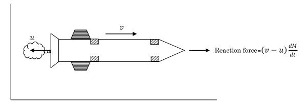
Motion of rocket is an example of system of variable mass. When the fuel in the combustion chamber of a rocket is burnt, pressure inside the chamber increases. Hence the hot gases inside the combustion chamber are ejected from the rocket in the form of a gas jet with high velocity in backward direction through a nozzle. Hence mass of the rocket decreases gradually due to the ejected gases and its velocity increases.
