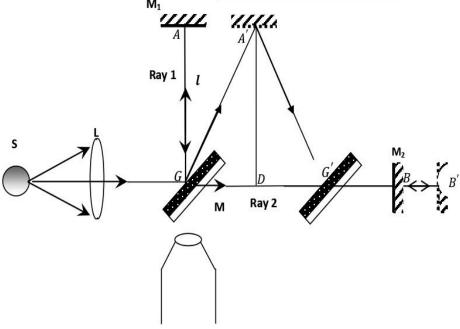
Aim: Aim of Michelson-Morley experiment is to determine the velocity of Earth relative to Ether.
