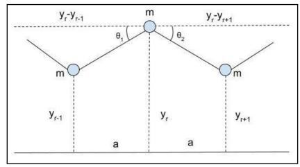
Consider a stretched elastic spring containing 'N' identical particles each of mass 'm' separated by a distance 'a' from each other. The total length of the string is (n+1)a. As shown in figure, let  $Y_r$ ,  $Y_{r-1}$  and  $Y_{r+1}$  be the displacements of  $r^{th}$ ,  $(r-1)^{th}$  and  $(r+1)^{th}$  particles.
